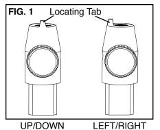
Select which adapter to use according to personal preference and work style. One adapter will allow the QC Tool Holder locating tab to be either UP or DOWN. The other adapter will allow the locating tab to be either in the LEFT or RIGHT position (FIG. 1).
