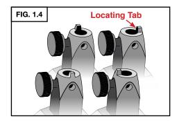
The Locating Tab may be oriented at 90° positions as needed to align the graver top with the EasyGraver Sharpening Fixture top.
