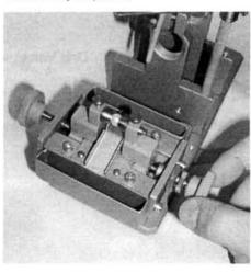
When using the Pearl Drill, the drill bit is stationary and you move the bead into the bit. This is done by sliding the Drilling Handle back and forth.
