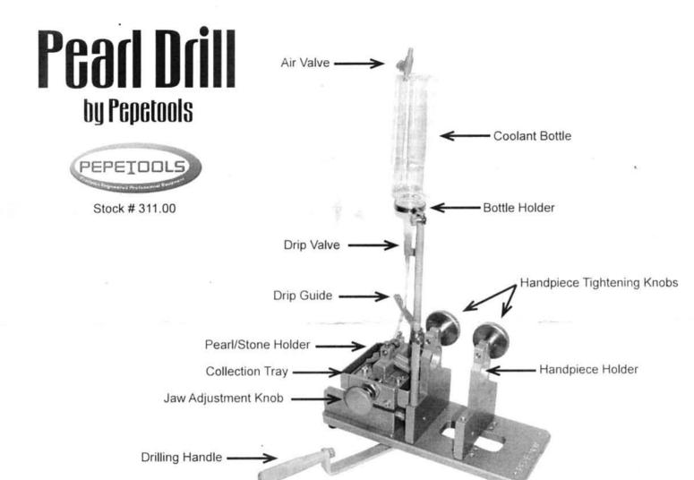
The new Pepetools Pearl Drill can be used to drill pearls or stone beads. It is made for use with a Foredom Flexshaft with a #30 handpiece. The unit includes The Pearl Drill, an optional drip cooling system and a set of 5 diamond core drills.
