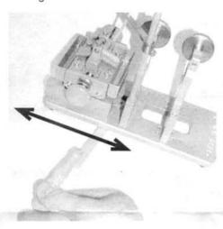
The Pearl drill is designed to make drilling from either side of the bead easy to do. To turn the entire holding table a full 360 degrees, start by pushing the Drilling Handle all the way to the end of its reach.
