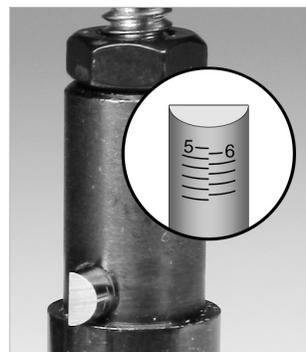
**4. INSTALL THE BORING BIT** To remove the wing blade from the reamer, loosen the locking nut with an adjustable wrench and then loosen the plastic knob by hand. Remove the wing blade and replace it with the boring bit. Position the bit as shown in the photo at left, lining up the desired size marking with the edge of the reamer. Size markings on the boring bit correspond to US standard ring sizes 5-15. *Tighten the boring bit by following the procedure in step 2.*
