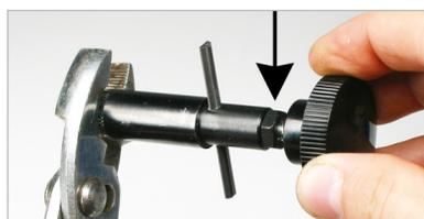
**2. TIGHTEN THE BLADE** Holding the knurled end of the tool with pliers, tighten the plastic knob firmly by hand. To prevent the knob from working loose during use, tighten the locking nut (indicated by the arrow in the photo at left) with an adjustable wrench.
