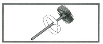
Discs must be mounted so as to rotate as shown in picture.
